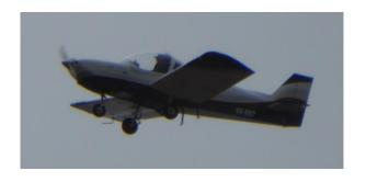
A subsequent flight enabled Lyndon to investigate the flight characteristics more fully with stalls in a variety of configurations. Half flap resulted in a stall speed of about 40 knots. The plane is over-propped at present as in 5 & L only 2400 rpm and 90 knots could be achieved. Some experimentation with
