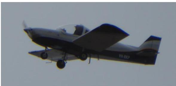
A subsequent flight enabled Lyndon to investigate the flight characteristics more fully with stalls in a variety of configurations. Half flap resulted in a stall speed of about 40 knots. The plane is over-propped at present as in S & L only 2400 rpm and 90 knots could be achieved. Some experimentation with
